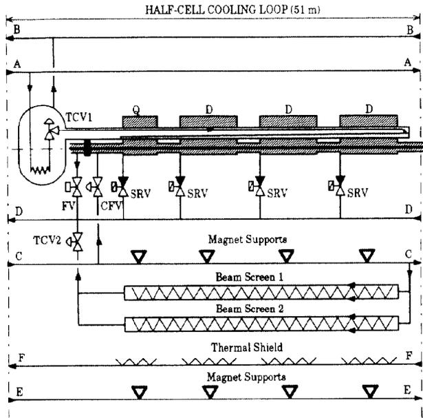
Figure 5 The elementary cryogenics loop.
