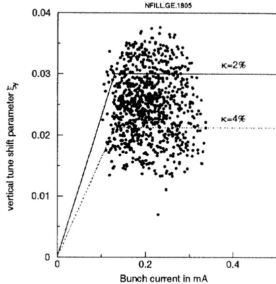
Figure 3:  $\xi_y$  dependence on current in Pretzel operation 1993. The expected behaviour for emittance ratios of  $\kappa = 2$  and 4 % is also shown.
