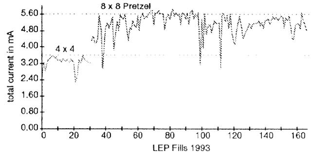
Figure 1: Total accumulated intensity at 20 GeV injection energy per fill in 1993
