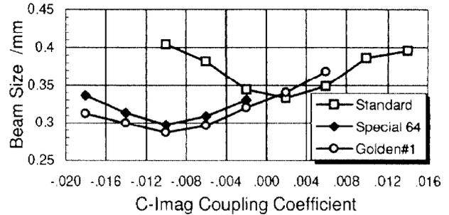
Figure 6: The Variation of Beam Size with the Imaginary Coupling Coefficient and Orbit Correction Strategy.
