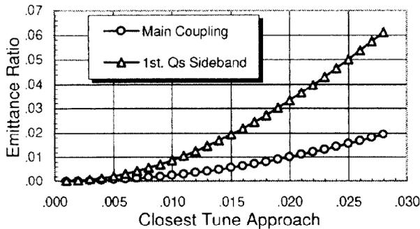
Figure 5: Emittance Ratio vs. Closest Tune Approach for Main Coupling and the 1st Qs Sideband Resonances.
