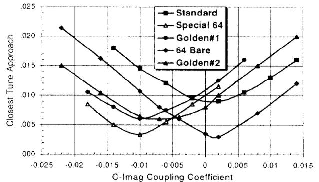
Figure 4: Coupling Curves for Various Vertical Orbit Correction Strategies.
