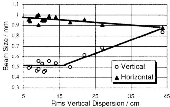
Figure 3: Horizontal and Vertical Beam Sizes, Measured at the BEUV as a Function of rms. Vertical Dispersion
