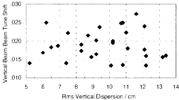
Figure 2: Beam-Beam Tune Shift vs. Vertical Dispersion
