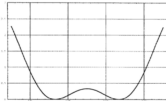
Figure 2: Beam loading enhancement factor  $B$  versus the HOM frequency  $f_{\text{HOM}}$  for  $s = 35\lambda_{\text{RF}}$  and  $k = 3$
