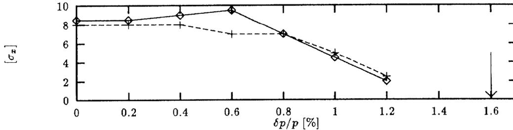
Figure 1: Comparison of the dynamic aperture with (solid line) and without (dashes) the sextupoles of the mid-arc bumps. This study was made on the physics optics used in 1993 with no radiation effects and the bumps were actually turned off. The limit of the RF bucket is shown at  $\delta p/p = 1.6$  %
