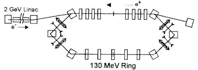
Figure 1: Possible layout of an asymmetric  $\phi$  factory using a linac and a storage ring.
