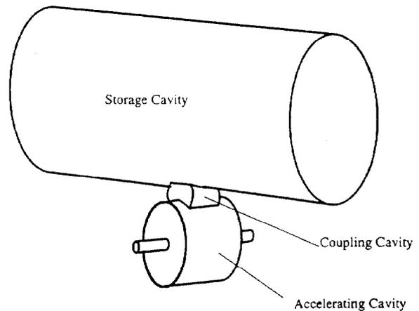
Fig. 3. A schematic view of ARES.
