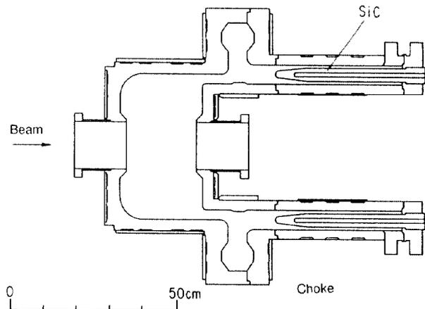
Fig. 4. Accelerating cell of ARES.
