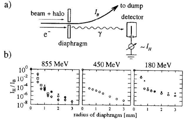
Figure 2: a) Schematic setup and b) results of beam halo measurements at different runs (different symbols).
