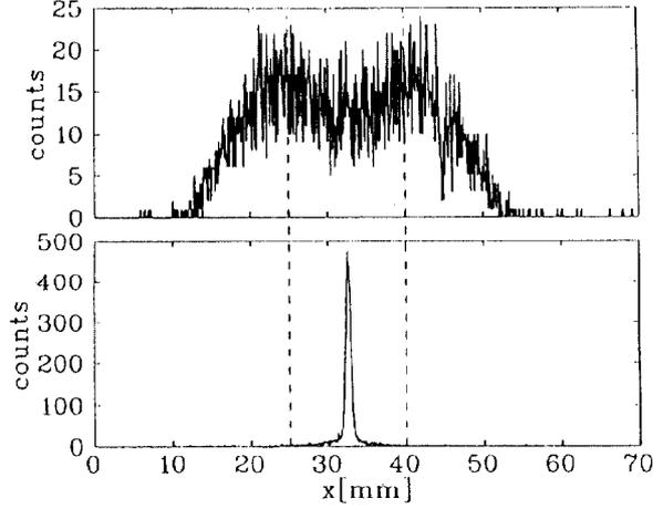
Figure 3: Measured beam profile for  $^{12}\text{C}^{6+}$  ions after multiturn injection (top) and after electron cooling for 1.5 s (bottom).
