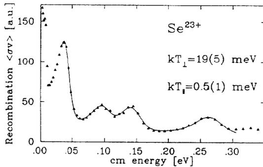
Figure 1: Dielectronic recombination rates for  $^{80}\text{Se}^{23+}$  ions.
