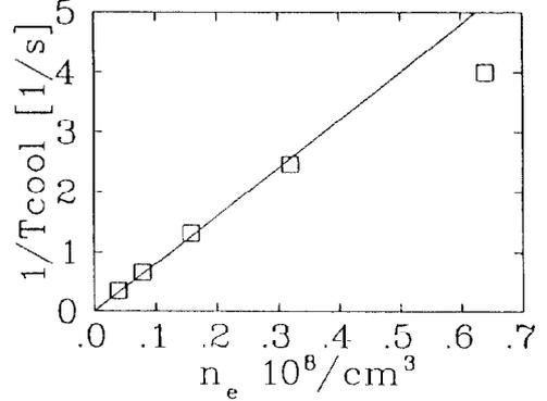
Figure 4: Measured inverse cooling time for  $^{32}\text{S}^{16+}$  ( $E=11.4$  MeV/u) as a function of electron density.
