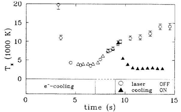
Figure 2: Evolution of the horizontal beam temperature observed with and without longitudinal laser cooling after electron precooling.
