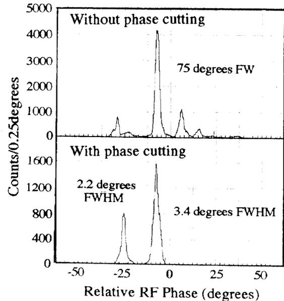
Figure 3: External beam phase distributions for the 10 MeV protons accelerated using the second harmonic at a RF frequency of 14.97 MHz. The initial beam intensity was reduced with the attenuators. Phases are relative, and zeros are not absolute.
