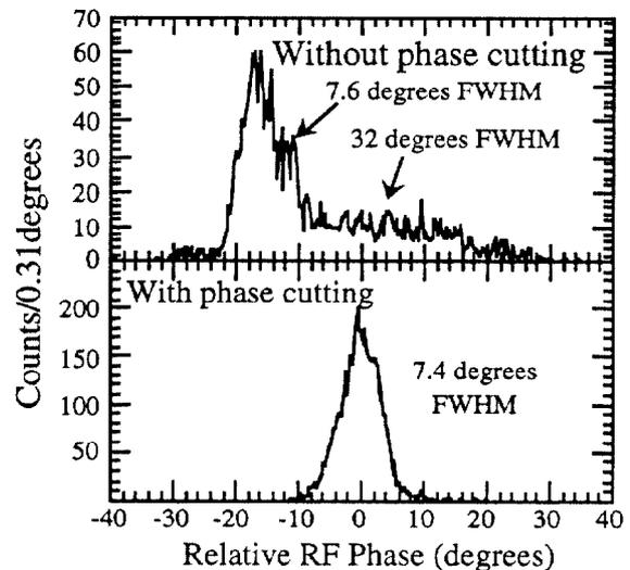
Figure 4: External beam phase distributions for the 70 MeV protons accelerated using the first harmonic at a RF frequency of 18.919 MHz. Phases are relative, and zeros are not absolute.
