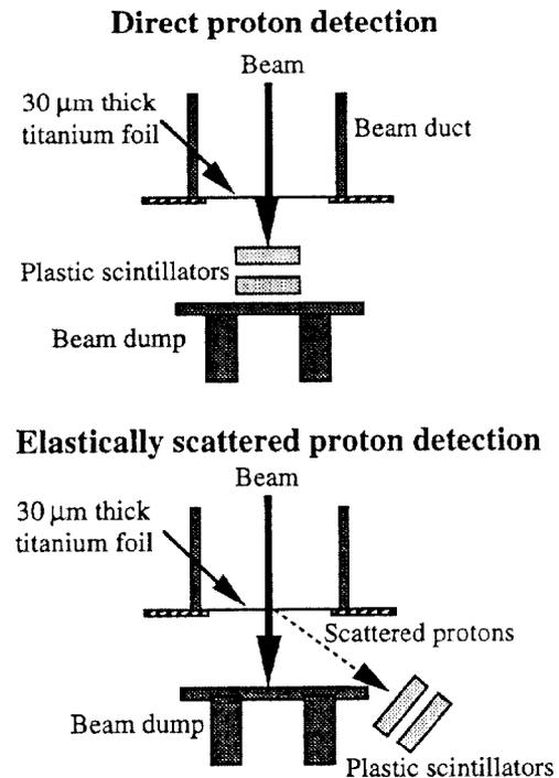
Figure 1: Schematic layouts of the measuring systems for the direct proton and elastically scattered proton detection.
