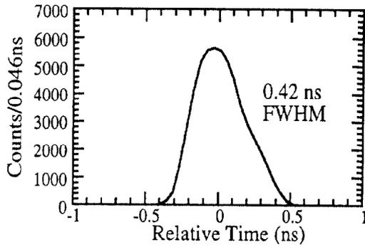
Figure 2: Time resolution of the plastic scintillators measured with a 70 MeV proton beam. The peak width of 0.41 ns FWHM gives a time resolution of 0.12 ns.
