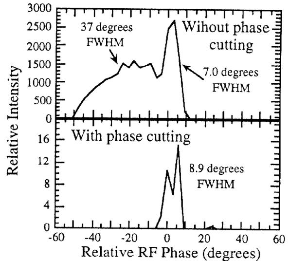
Figure 6: Calculated external beam phase distributions for the 70 MeV protons with and without phase cutting. The spectrum for the beam without phase cutting was fitted using two independent Gaussian functions.
