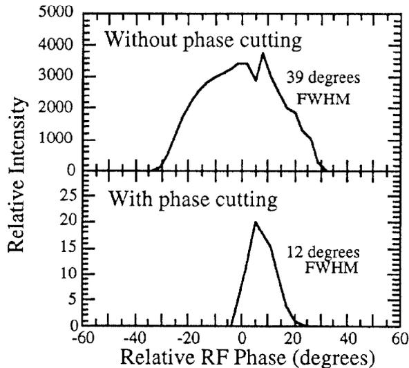
Figure 5: Calculated internal beam phase distributions for the 70 MeV protons with and without phase cutting. Peak widths were evaluated using a Gaussian function.
