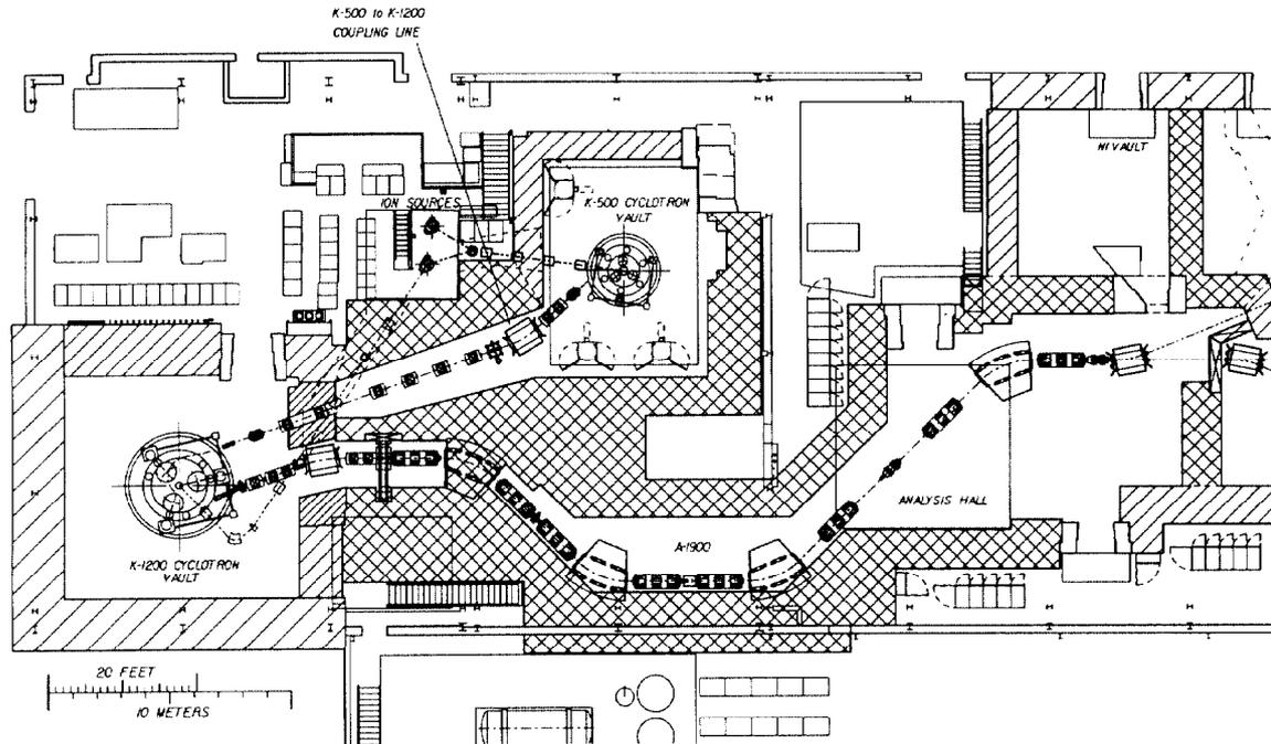
Figure 1: Proposed new accelerator area of the National Superconducting Cyclotron Laboratory.
