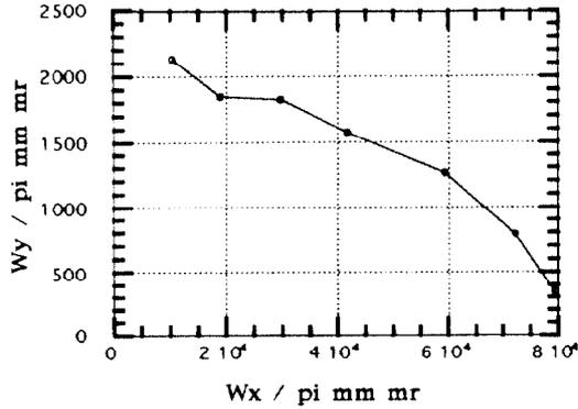
Figure 1: Dynamic aperture for the 2.5 GeV FFAG. The tunes are  $Q_x=4.78$ ,  $Q_y=3.29$  at a field index of  $k=16.69$
