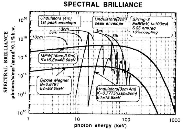
Fig. 4. Spectral Brilliance from the SPring-8 Light Sources
