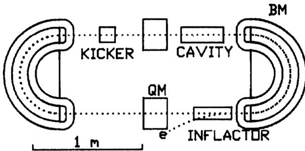
Figure 6: Schematic drawing of the storage ring
