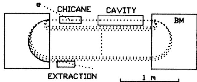
Figure 4: Schematic drawing of the race track microtron
