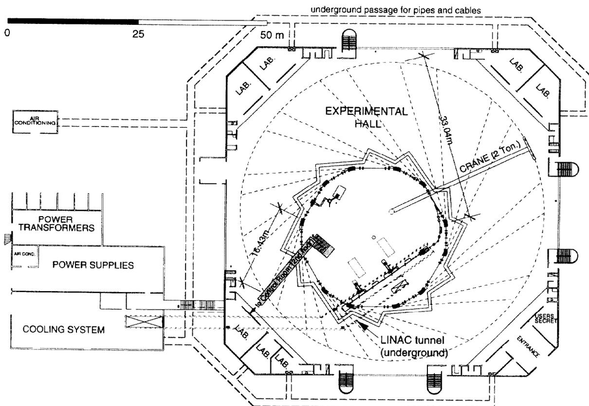
Figure 1: Main Building with the storage ring and experimental hall, on the ground floor, and underground LINAC.
