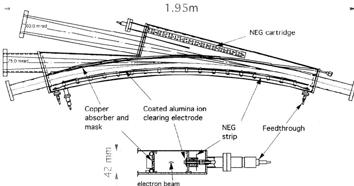
Figure 3: Bending magnet vacuum chamber.
