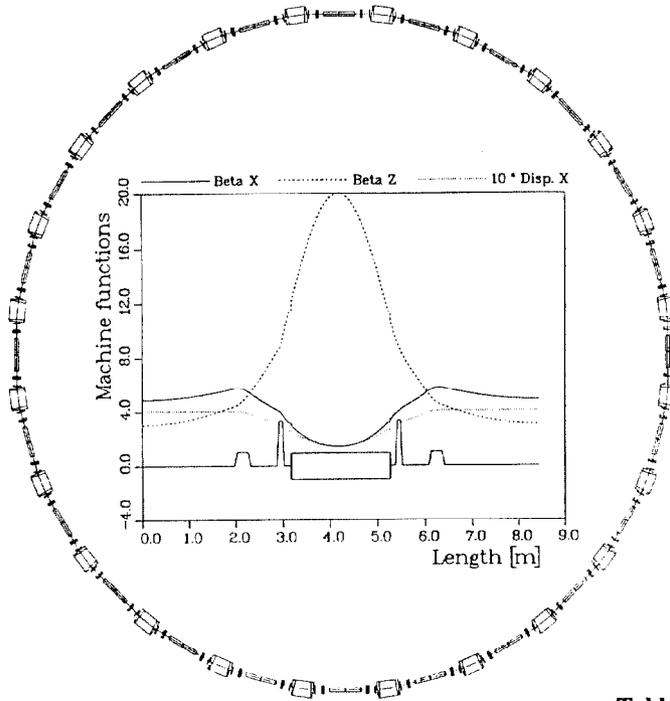
Figure 1: A bird's eye view of the storage ring with 24 IDs. Inserted are the horizontal and vertical beta functions and the dispersion of the unit cell.
