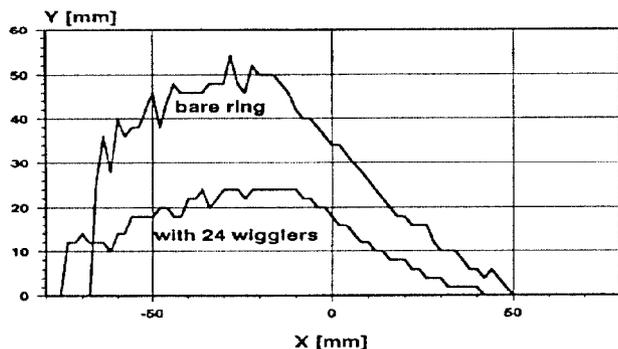
Figure 3: The dynamic aperture for the bare ring and with 24 wigglers.
