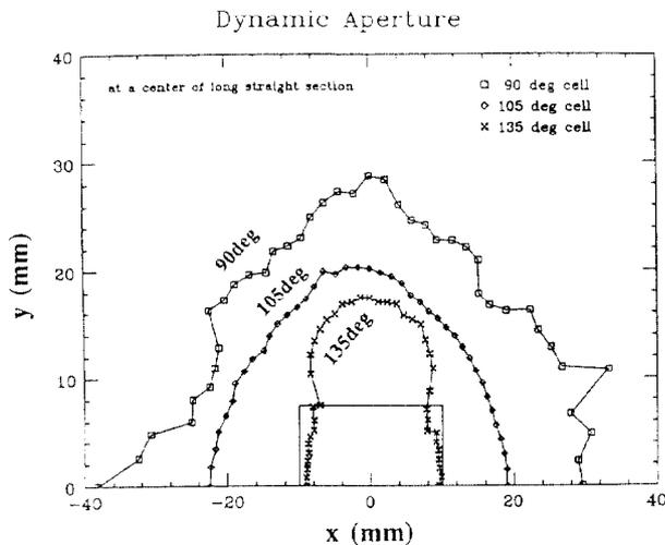
Figure 6. The dynamic aperture of the low emittance lattice. Those of 90, 105 and 135 degree lattice are shown. The square in the figure indicates the horizontal aperture required for injection and the vertical physical aperture determined from the narrow vacuum chambers at the insertion devices. The results without machine errors and energy deviation are shown here. With these errors, the dynamic aperture is reduced typically by 20%
