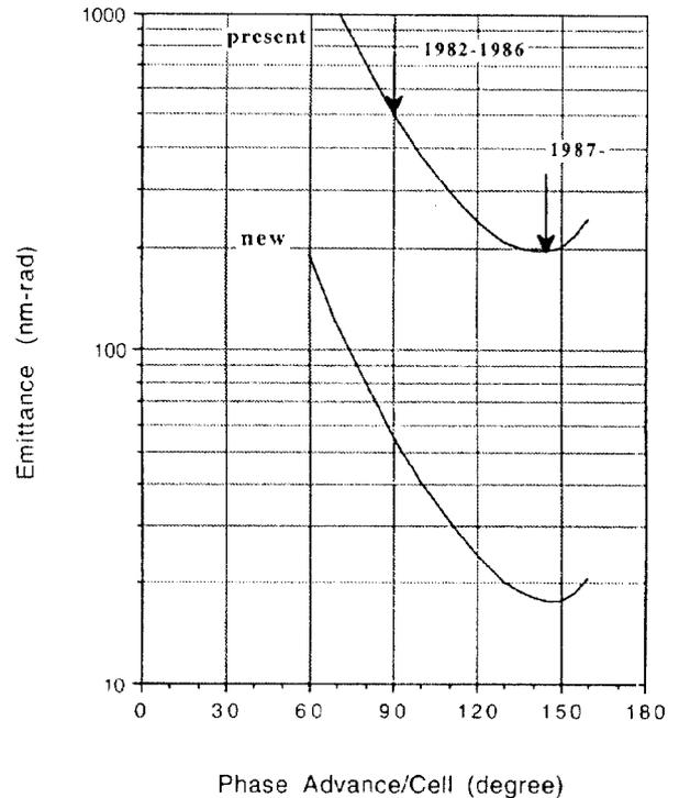
Figure 1. Horizontal betatron phase advance vs. Emittance. It is assumed that the whole ring consists of normal cells only. The upper curve is for the present lattice and lower is the new one (see Figure 2 and 3). The operating point before and after the 1986 low emittance program is shown by arrows.
