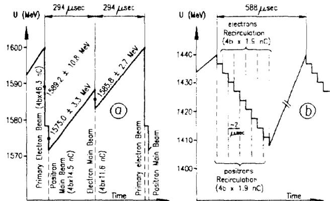
Fig. 2: Compensation of beam loading in the injector (a) and in the booster (b) linacs:
