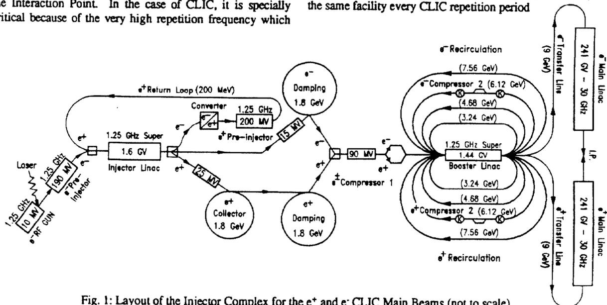
Fig. 1: Layout of the Injector Complex for the  $\text{e}^+$  and  $\text{e}^-$  CLIC Main Beams (not to scale)
