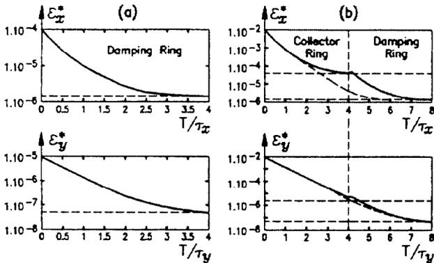
Fig. 3: Damping of the normalized transverse emittances of the electron (a) and positron (b) beams as a function of the circulating time,  $T$ , normalized to the damping time,  $\tau_{x,y}$ .
