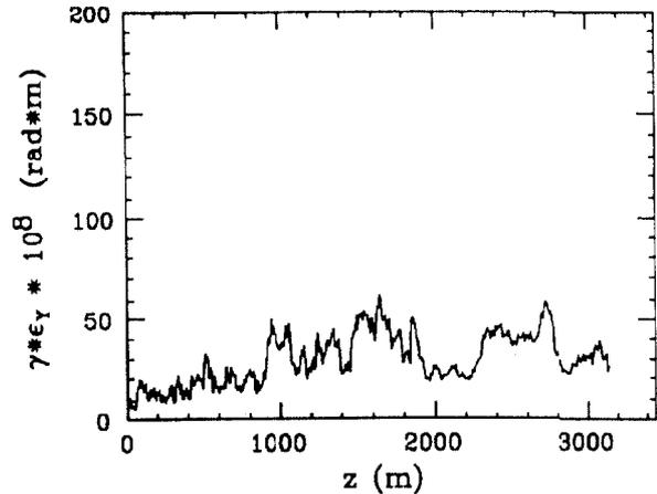
Figure 7. Vertical emittance blow-up with 30 iterations more in the last kilometre, with one pick-up every 2 metres.
