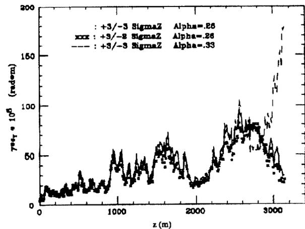
Figure 4. Vertical emittance blow-up along the linac with the 'new scaling' strategy and alignment r.m.s. errors of  $10 \mu\text{m}$  on quadrupoles, pick-ups, and cavities.
