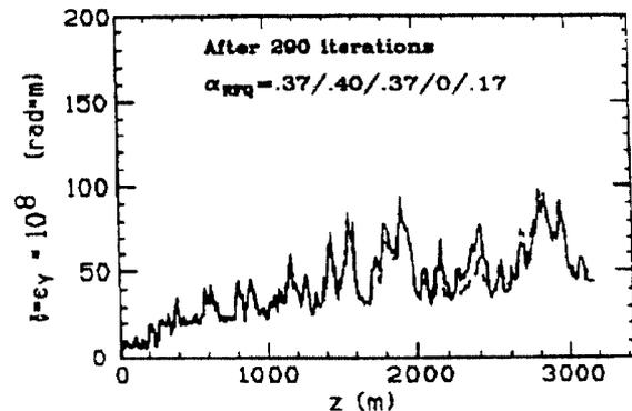
Figure 1. Vertical emittance blow-up along the linac with a scaling according to  $(E/E_0)^{1/2}$  and alignment r.m.s. errors of 10  $\mu\text{m}$  on quadrupoles, pick-ups, and cavities.
