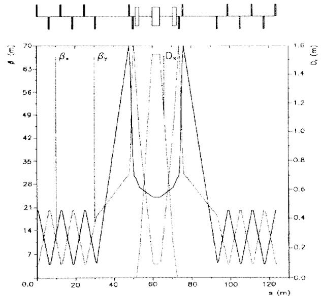
Figure 2. Optics functions of the low-energy compressor.
