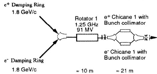
Figure 1. Low-energy bunch compressor.
