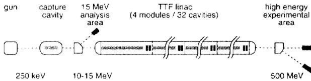
Figure 1: Schematic layout of the TTF linac. The overall length of the installation at DESY [10] amounts to  $\approx 85$  m; the drawing is not to scale.
