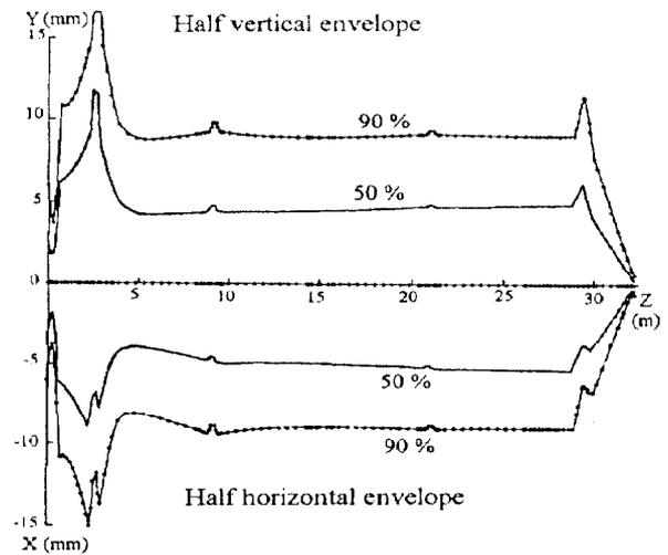
Figure 2. Beam envelopes without beam loading effect
