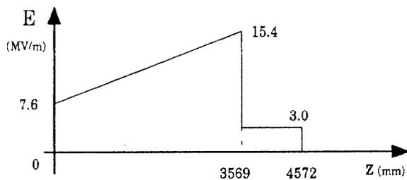
Figure 4. Electric field shape in accelerating sections with LIPS
