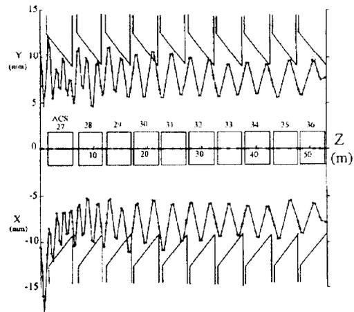
Figure 5. Beam envelopes with the new optics
