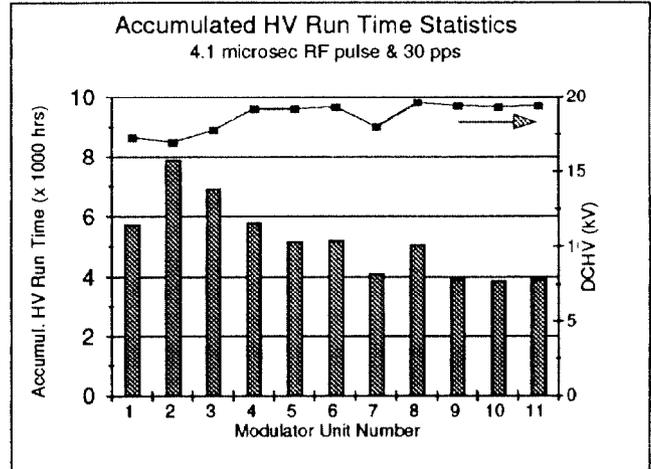
Fig. 1: Accumulated HV run time for modulators and DC high voltages for the operation on May 19, 1994.
