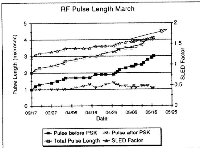
Fig. 3: RF pulse width change during the commissioning.
