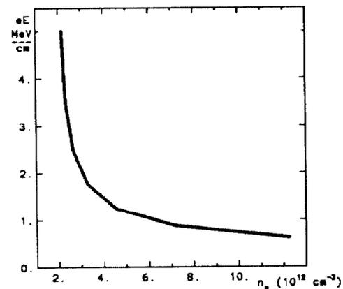
Fig.2. The acceleration rate as a function of the plasma density; beam current density is fixed at  $5 \text{ kA/cm}^2$
