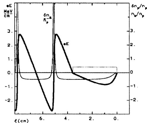
Fig.1. The distributions of the perturbed plasma density,  $\delta n_p/n_p$ , and the longitudinal electric field,  $eE$ , behind electron bunch (the bunch itself is shown with the dotted line); beam and plasma parameters see in the text.
