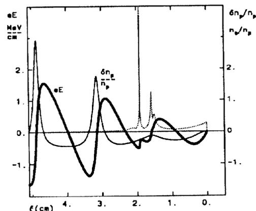
Fig. 3. Same as in Fig.1 but after a pathlength of  $72.5 \text{ cm}$  in the plasma of the density of  $3.3 \cdot 10^{12} \text{ cm}^{-3}$ ; initial length of the bunch is  $1.7 \text{ cm}$ , initial electron density is  $1 \cdot 10^{12} \text{ cm}^{-3}$ .
