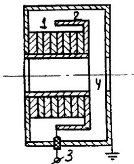
Fig. 5. An injector ERA accelerating device
