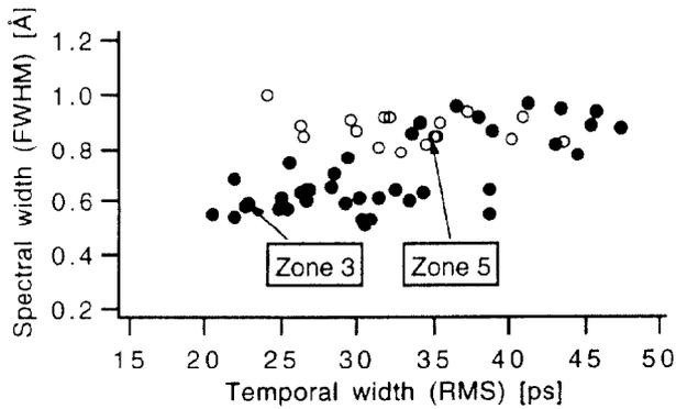
Figure 6. Temporal and spectral width of the laser micropulse in zones 3 and 5.
