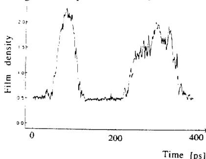
Figure 3. Temporal distribution of the laser micropulse observed by the streak camera. Vertical axis corresponds to the logarithm of luminosity and two micropulses are taken on one film.
