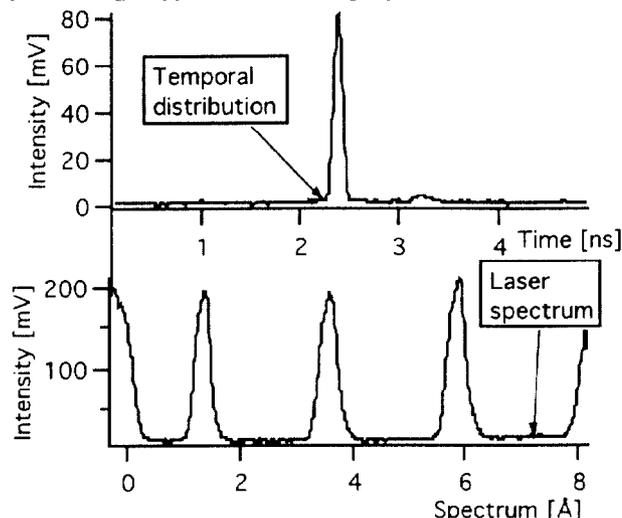
Figure 4. Temporal distribution of the laser micropulse and laser spectrum, which are simultaneously obtained by the dissector and the scanning Fabry-Perot respectively.
