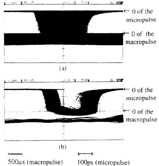
Figure 7. Laser micropulse and macropulse, (a) with the feedback off, and (b) with the feedback on. The upper channel shows the laser micropulse and its jitter, and the lower channel shows the laser macropulse. Data are accumulated by an oscilloscope for one minute. All signals are negative.
