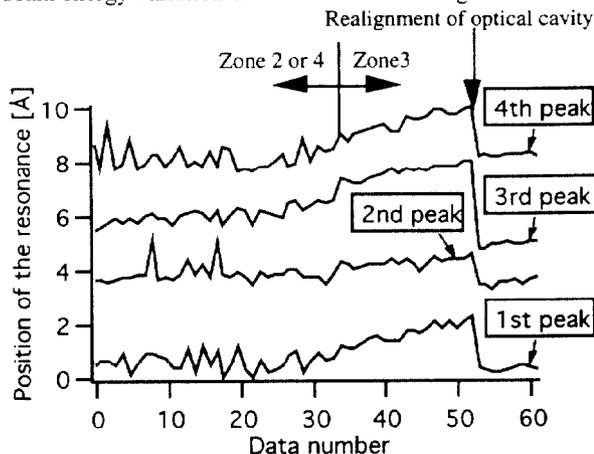
Figure 5. Drift of the lasing wavelength. Data number corresponds to time arbitrarily. One scan includes four resonant points in this case.
