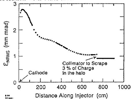
Figure 2: LCLS RF Gun Injector  $\epsilon_{n,rms}$  for 1 nC, 10 ps FWHM Beam (Parmela simulations)
