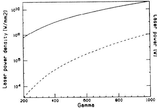
Figure 4: Laser power density  $\mathcal{P}$  vs  $\gamma$  and laser power  $P_L$  vs  $\gamma$ .
