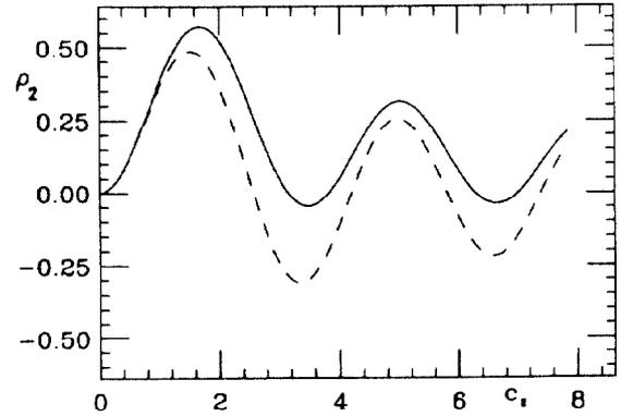
Figure 5: Amplitude oscillation of the harmonic component  $\rho_2$  in an isochronous transport line (continuous line) and in a dispersive one (dashed line).
