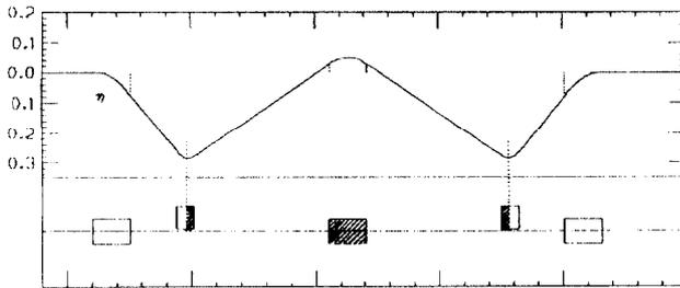
Figure 1: Schematic of magnetic transport line and dispersion function  $\eta$  for bunching. Dashed elements are to be included for the isochronous transport line which requires  $\eta < 0$  in the middle magnet.
