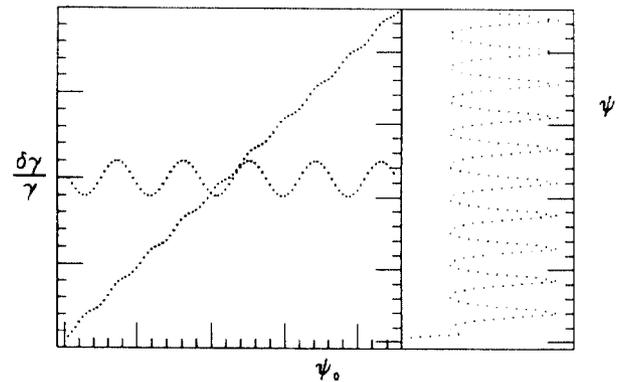
Figure 2: Energy modulation at  $\psi_o$  and longitudinal position  $\psi$  after an isochronous transport line. The resulting longitudinal density modulation of an initially monoenergetic beam is shown in the vertical projection on the right side.
