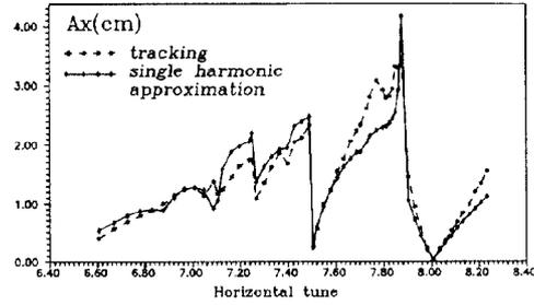
Figure 4: Horizontal DA versus unperturbed betatron tune. Tracking and 5th order prediction.
