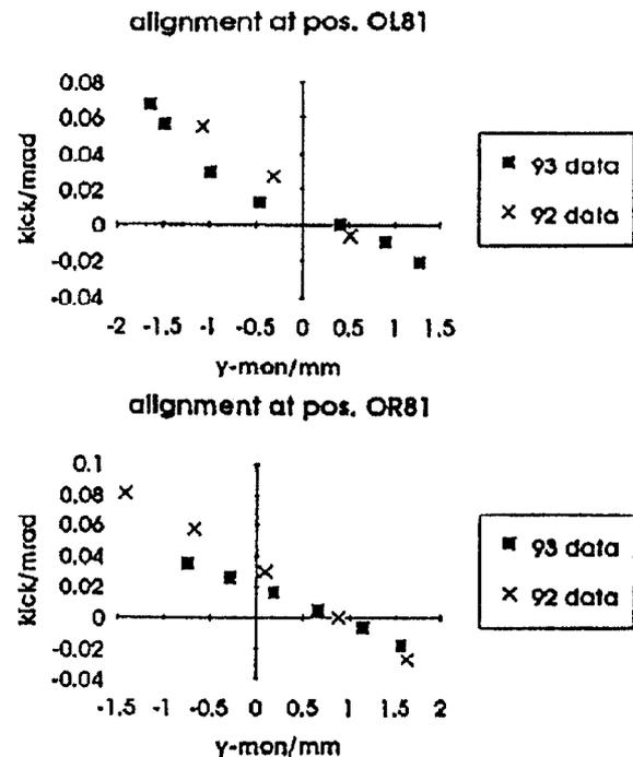
Figure 1: Results of the beam-based alignment test measurements for quadrupoles and monitors at position OL81 and OR81 in the straight section East of HERA-e. Shown are the kicks obtained from the difference orbit for various values of the nominal orbit in the monitor. The offset of the monitor with respect to the quadrupole is given by the x-axis intercept of a straight line fitted to the data
