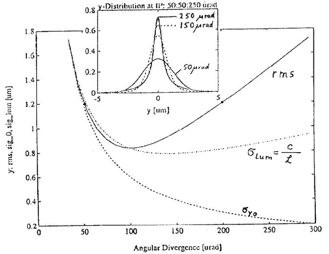
Figure 3: Vertical Spot Size vs Angular Divergence
