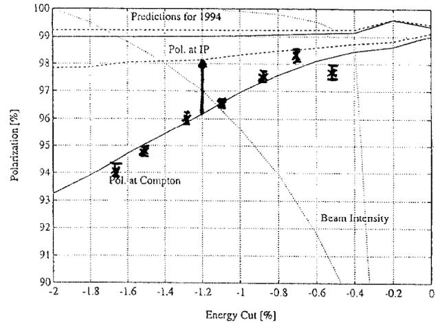
Figure 5: Correlation of Polarization versus Collimator Position.
