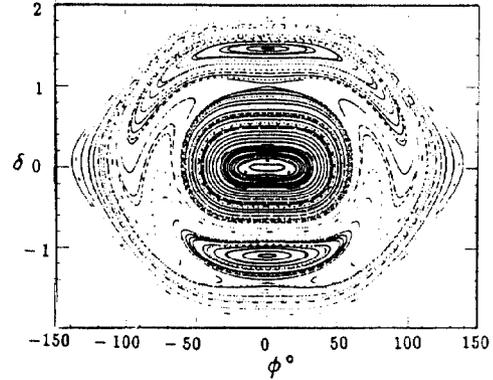
Figure 5: Poincaré surface near the bifurcation of the  $n = 1$  resonance with  $\alpha = 1^\circ$  and  $\frac{\nu_m}{\nu_s} = 0.9$ .
