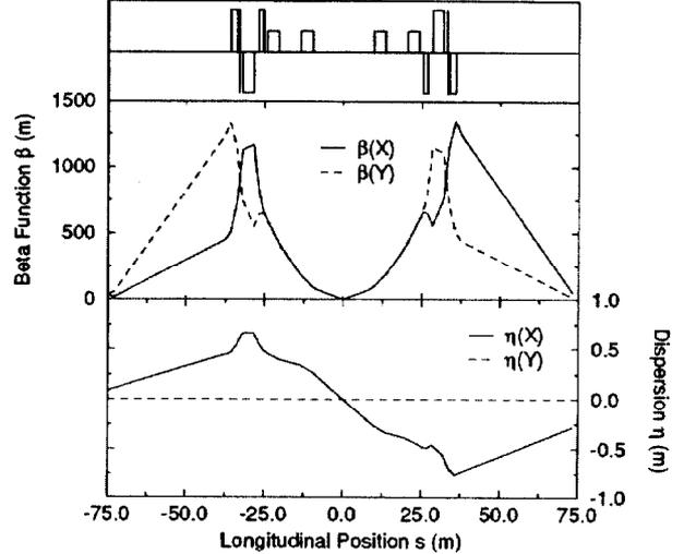
Figure 1: Optical functions near the 8 o'clock IR and the PHENIX experimental area for a  $\beta^* = 1$  m lattice. Longitudinal position is measured from the interaction point. The positions of IR quads 1-3, IR skew quad correctors (next to IR quad 3), and the DX and D0 dipoles are also shown.
