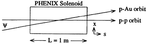
Figure 2: Orbit through the PHENIX solenoid, for proton-proton and proton-gold collisions. The orbit skew angle is  $\psi = 3.85\text{ mrad}$ .
