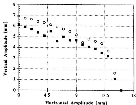
Figure 5. Dynamic aperture by simulation with (white) and without (black) insertion devices at minimum gaps
