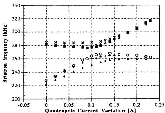
Figure 2. Measurement of the difference coupling resonance
