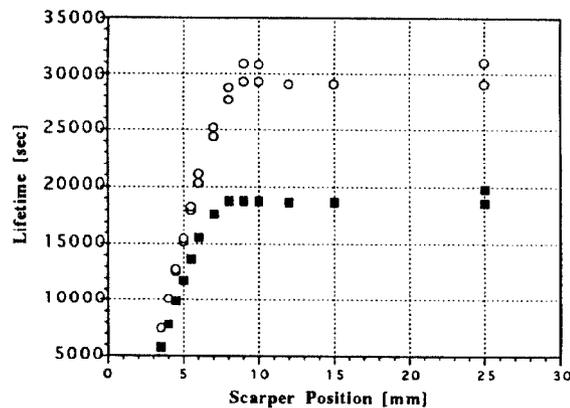
Figure 4. Vertical dynamic aperture measurement with (black) and without (white) insertion devices closed at minimum gaps.
