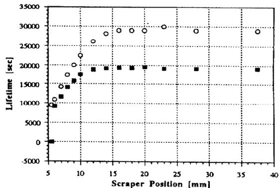
Figure 3. Horizontal dynamic aperture measurement with (black) and without (white) insertion devices closed at minimum gaps.
