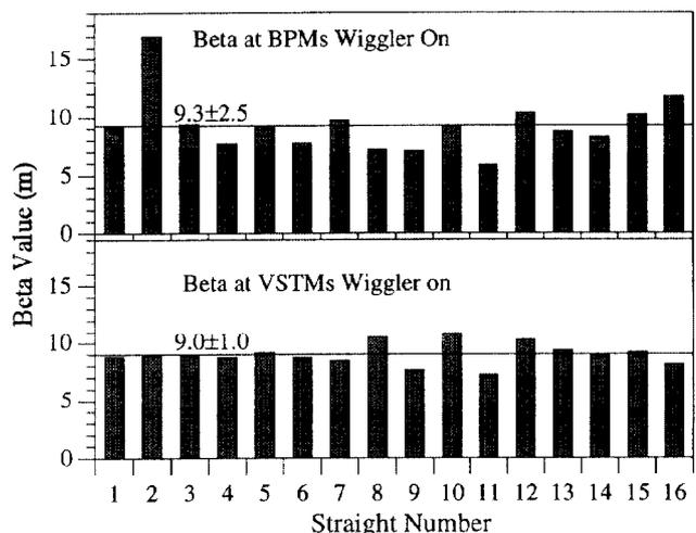
Fig 2 Beta values at BPM and steering magnet illustrating result of BPM response error.
