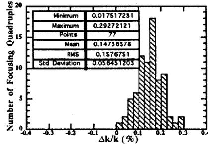
Figure 1: Strength Errors of QF magnets.
