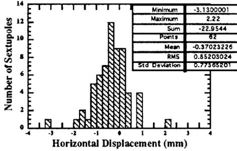
Figure 3: Horizontal Alignment Errors of Sextupoles.
