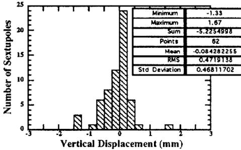
Figure 4: Vertical Alignment Errors of Sextupoles.
