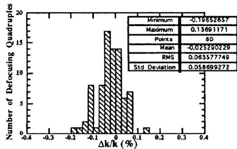
Figure 2: Strength Errors of QD magnets.
