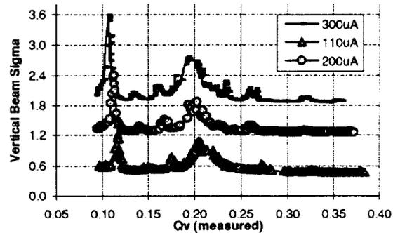
Figure 1. Vertical beam size (arbitrary units) as function of the measured vertical tune value.
