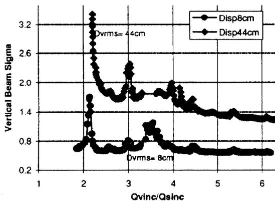
Figure 5. Tune Scans with Two Values of Dispersion
