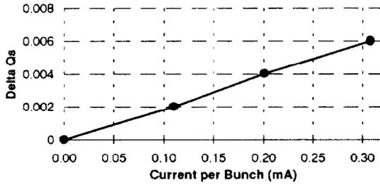
Figure 4. Incoherent synchrotron tune shift vs bunch current
