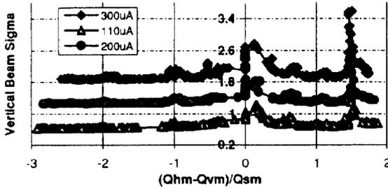
Figure 3. Tune scans at Different Bunch Currents
