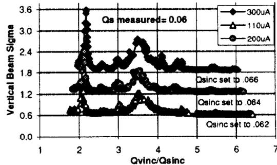
Figure 2. Tune scans at Different Bunch Currents
