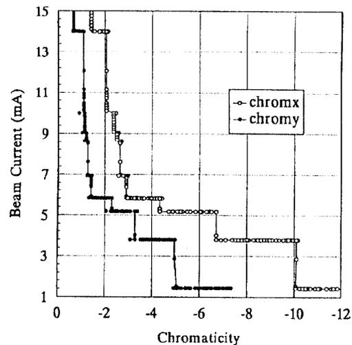
Fig. 3 The chromaticities knob vs. survival beam current for the case of the difference resonance tune setting.
