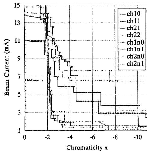
Fig. 4 The chromaticity x vs. survival beam current (please see the text for the conditions for different curves)
