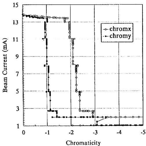
Fig. 2 The chromaticities knob vs. survival beam current for the case of the normal tune setting.
