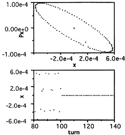
Fig. 2: An example of transverse deadbeat-control feedback
