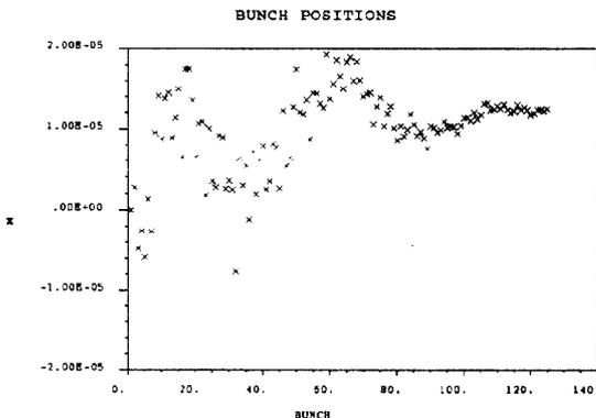
Figure 5: Position of the bunches at the end of the SBLC linac versus the bunch number. The dipole modes a damped  $Q = \text{profile}$ .
