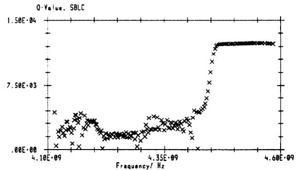
Figure 4:  $Q$ -values of the SBLC dipole modes versus their frequencies [4].
