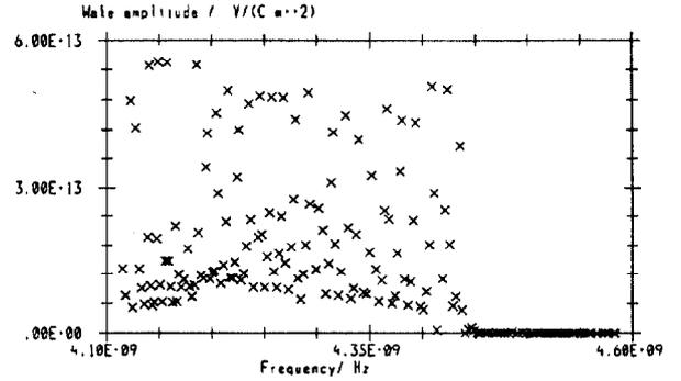
Figure 3: Amplitude of the wake potential  $W_m$  of the  $m = 1 \dots 180$  SBLC dipole modes versus their frequencies.
