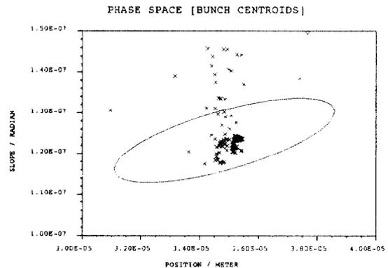
Figure 2: Vertical multi-bunch phase space, ( $y'$ ,  $y$ ) centroids of the TESLA bunch train. The multi-bunch one sigma ellipse is shown,  $Q_{ref} = 1.0 \cdot 10^5$ .
