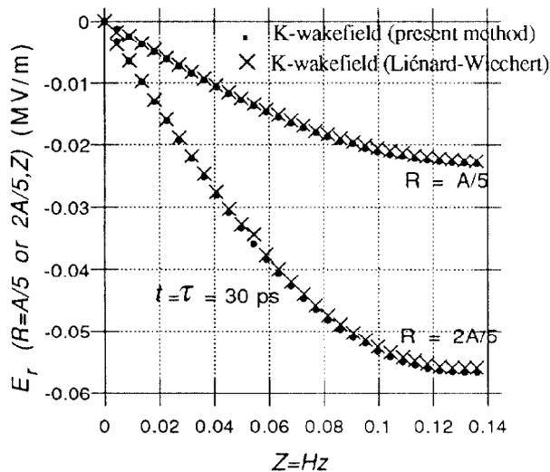
Fig. 4. On an exemple, comparaison between wakefields obtained by the present method or by Liénard-Wiechert's one
