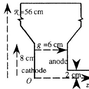
Fig. 1. Schematic of ELSA photoinjector
