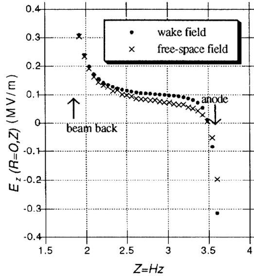
Fig. 3a  $E_z(R=0,Z)$  : wakefield and free-space field for  $t=t_g$ .
