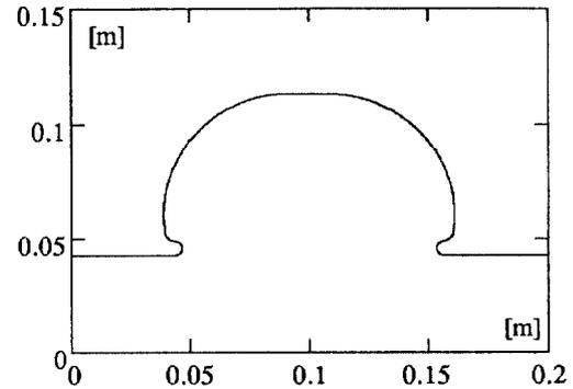
Figure 5. Nosecone high  $R_S$  cell.
