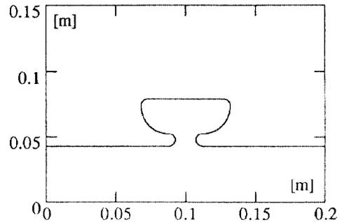
Figure 3. Nosecone 'single-mode' cavity.
