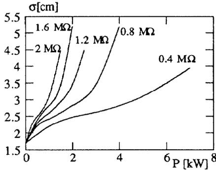
Figure 2. Bunch length versus dissipated power.
