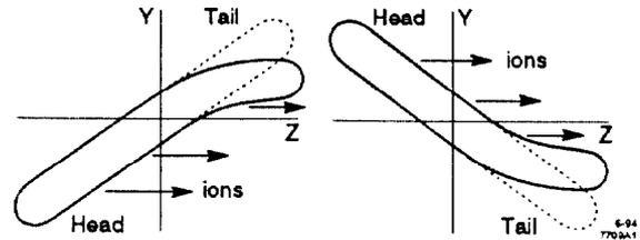
Figure 1: Schematic picture of resonant tail excitation for two different betatron phases.
