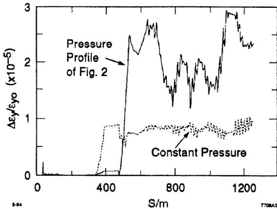
Figure 3: Relative increase of vertical emittance as a function of position along the arc for an average pressure of  $2.2 \times 10^{-5}$  torr. The two curves correspond to different pressure profiles.
