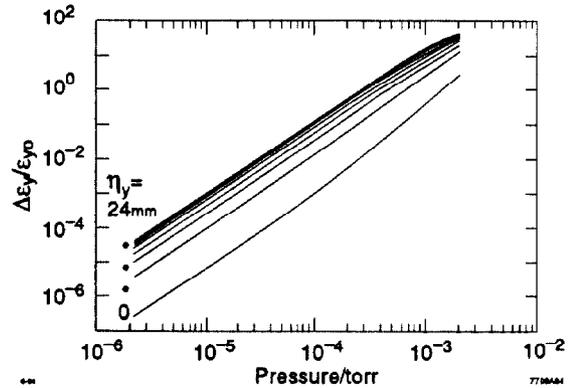
Figure 4: Relative increase of the vertical emittance along the entire arc as a function of the pressure, for different values of dispersion mismatch.
