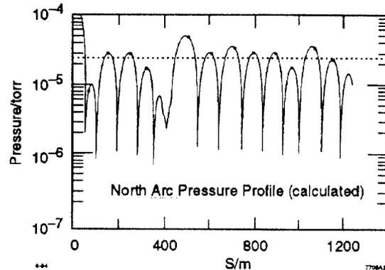
Figure 2: Pressure profile in the SLC north arc calculated according to [5]. The dips are the pump locations. The circles indicate newly installed vacuum gauges.
