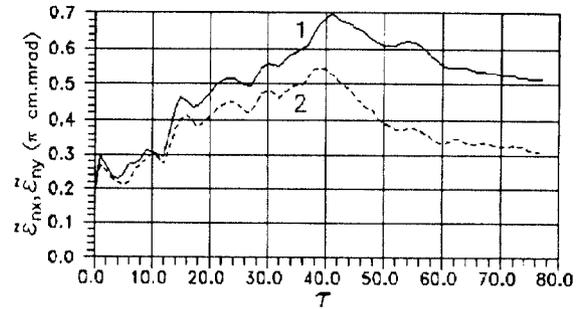
Figure 5: The normalized rms emittances  $\tilde{\epsilon}_{nx}$  (1),  $\tilde{\epsilon}_{ny}$  (2) vs the dimensionless longitudinal coordinate  $\tau$  at the beam injection without modulation in longitudinal velocities.
