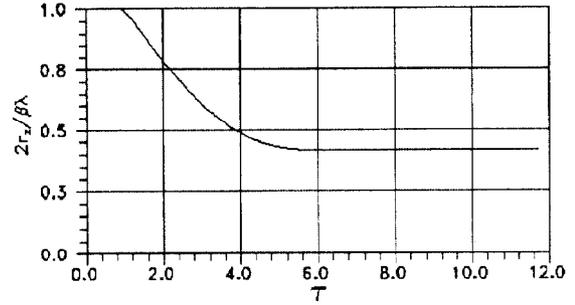
Figure 2: The relative bunch length  $2r_z/\beta\lambda$  vs the dimensionless longitudinal coordinate  $\tau$ .
