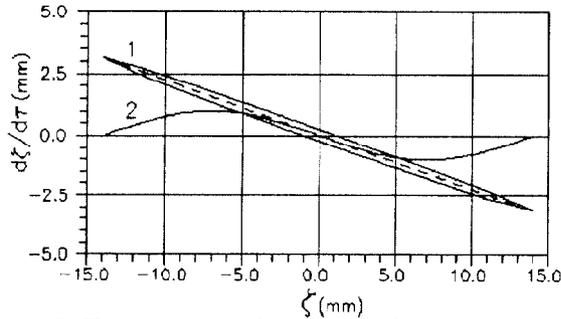
Figure 3: The representative ellipse (1) at the touch position of bunches and the phase portrait of matched beam (2) at the linac entrance for zero longitudinal emittance.
