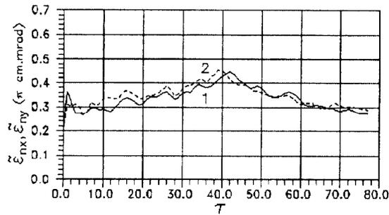
Figure 4: The normalized rms emittances  $\tilde{\epsilon}_{nx}$  (1),  $\tilde{\epsilon}_{ny}$  (2) vs the dimensionless longitudinal coordinate  $\tau$  at the beam injection with sinusoidal modulation in longitudinal velocities.
