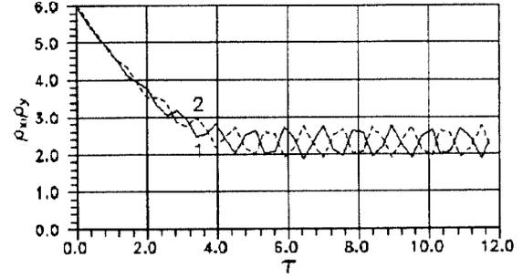
Figure 1: The normalized beam envelopes  $\rho_x$  (1),  $\rho_y$  (2) vs the dimensionless longitudinal coordinate  $\tau$ .
