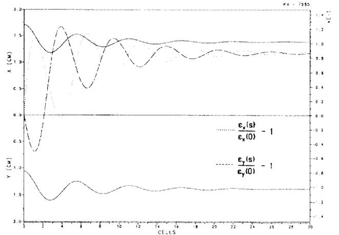
Figure 1: Envelopes and emittance growth functions of a mismatched beam passing through a Continuous Focusing Channel. (The scale on the right-hand side applies to the dimensionless emittance growth functions.)
