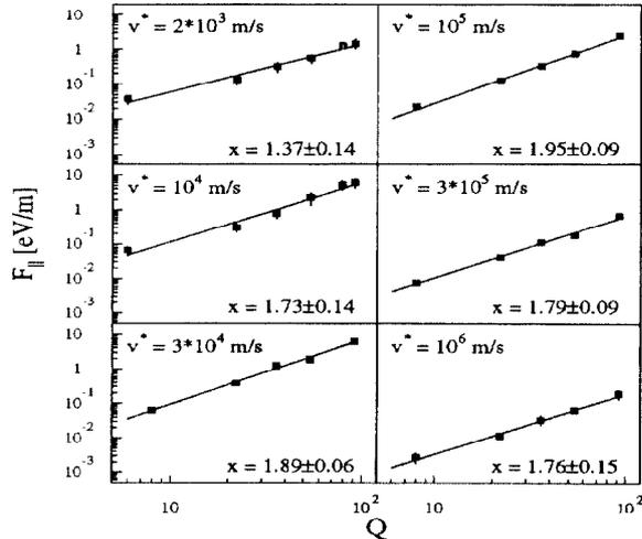
Figure 2: Cooling forces as a function of the ion charge. Relative velocity as indicated in the viewgraph. Data were fitted according to  $F_{\parallel} \propto Q^x$ .
