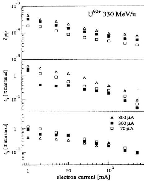
Figure 4: Momentum spread and emittances of a cooled  $U^{92+}$  330 MeV/u beam as a function of the electron current for three ion beam intensities.
