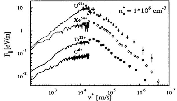
Figure 1: Cooling forces normalized to an electron density  $n_e^* = 1 \cdot 10^6 \text{ cm}^{-3}$  as a function of the relative velocity (typical kinetic energy 250 MeV/u).
