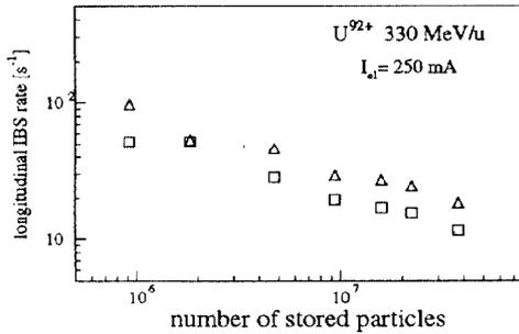
Figure 5: Calculated longitudinal intrabeam scattering rates for  $U^{92+}$  cooled with a 250 mA electron beam. Squares are calculated from [9], triangles from [10].
