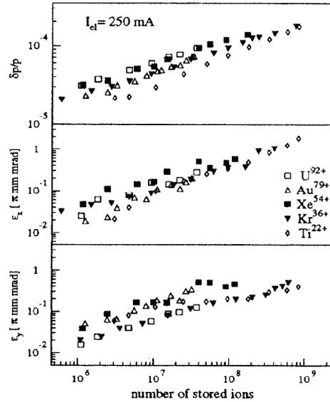
Figure 3: Momentum spread and emittances of a cooled heavy ion beams as a function of the number of stored ions.
