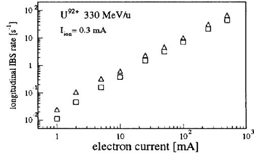
Figure 6: Calculated longitudinal intrabeam scattering rates for  $U^{92+}$  (300  $\mu$ A) cooled with varying electron current. Squares are calculated from [9], triangles from [10].
