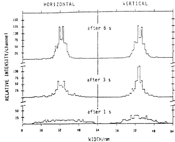
Figure 4: Horizontal and vertical  $H^0$  spectra of the cooled proton beam in COSY
