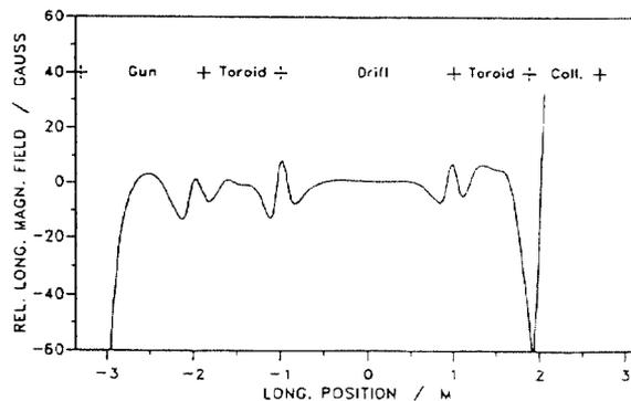
Figure 1: The longitudinal magnet field deviations at a level of 0.12 T.
