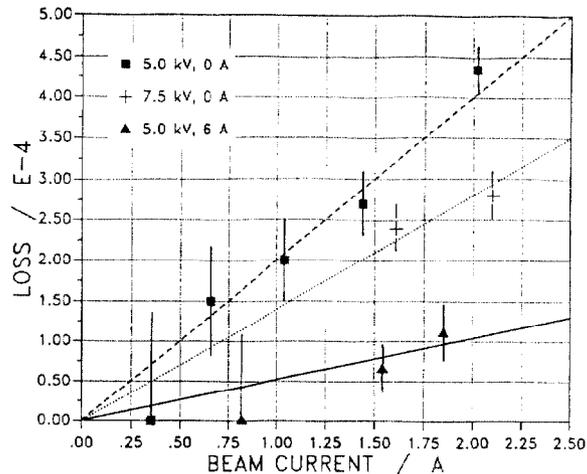
Figure 2: Electron loss as function of the electron current, varied are the collector anode voltage and the collector end coil current.
