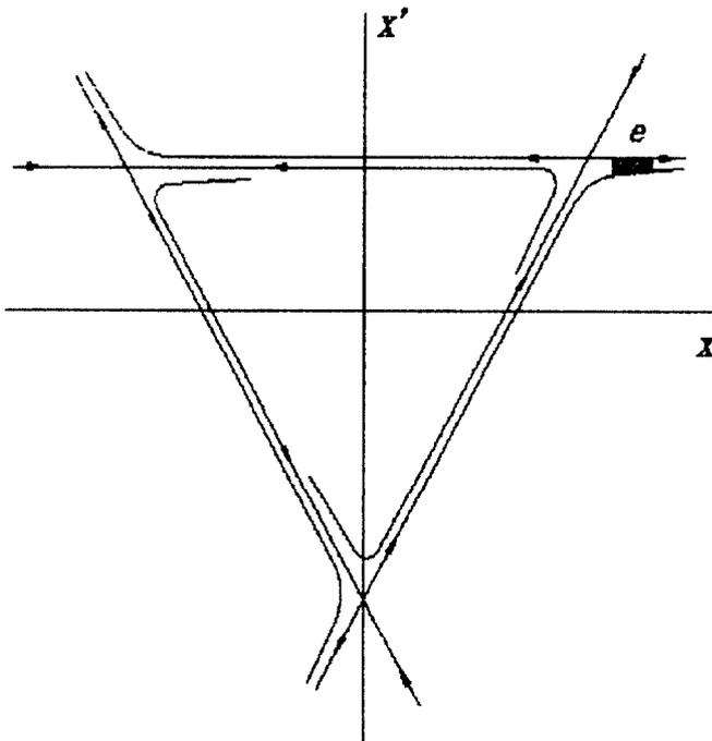
Fig.1. The quasiseparatrix of the resonance  $3\nu_x = m$ .
