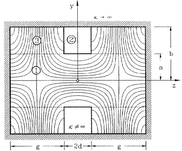
Figure 3: Two iris coupled resonators and electric field pattern for  $k_0 a = 1.73956$
