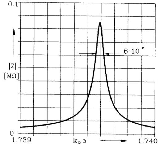
Figure 4: Absolute value of the impedance in the vicinity of resonance
