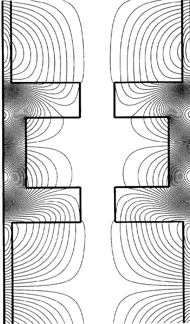
Figure 2: Field pattern in a tube with dielectric walls
