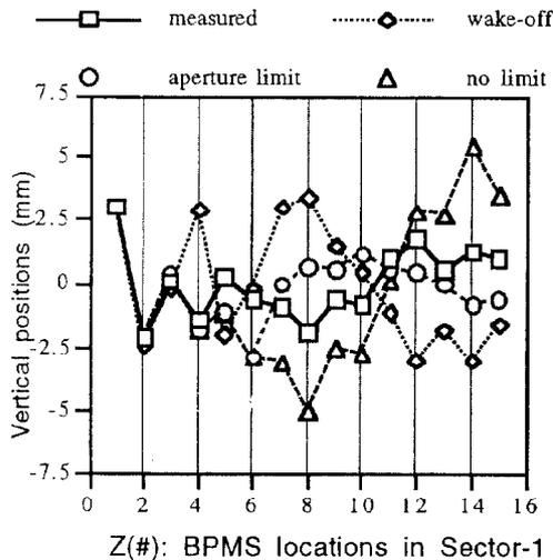
Figure 6. Simulation and measured results of beam trajectory versus BPMs.
